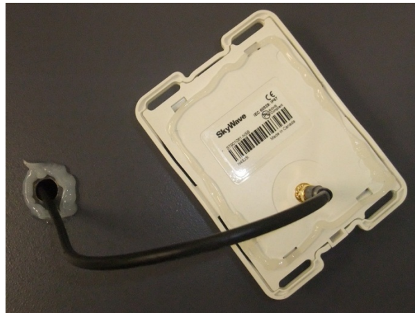
Figure 42: Apply Silicone to Hole in Asset
