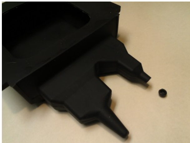
Figure 57: Cut Tip of RF Cable Portion
