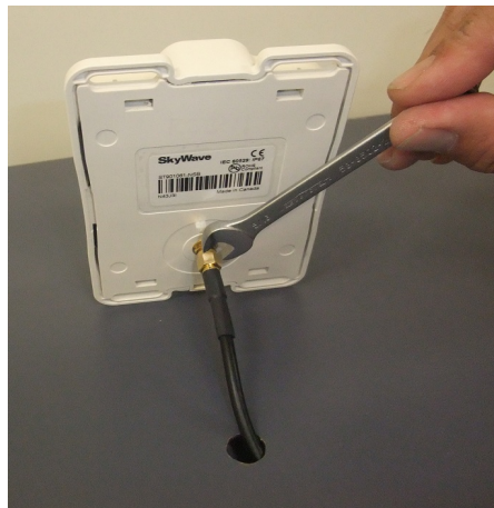
Figure 41: Attach Cable to Terminal
