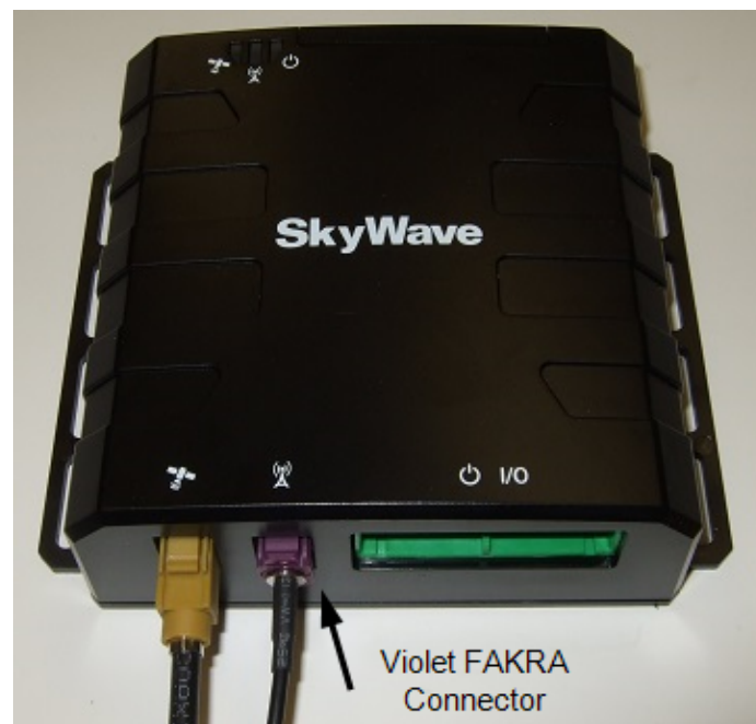
Figure 54: Connect the Cellular Antenna
