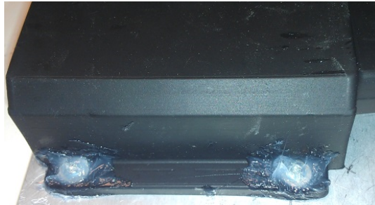
Figure 67: Apply Silicone to Hardware
