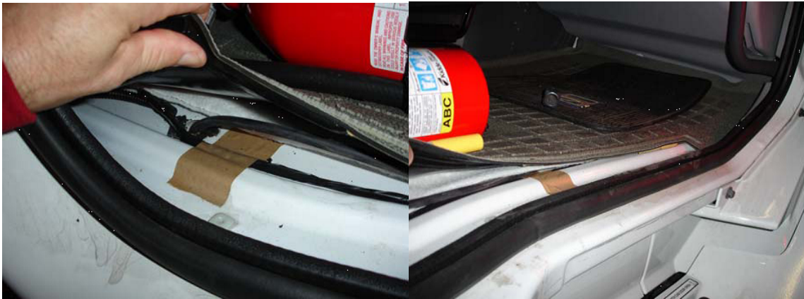
Figure 51: Sample Cable Placement in a Vehicle Cab
