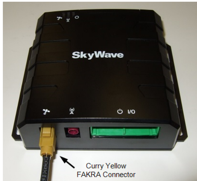
Figure 53: Connect the Remote Antenna (satellite antenna shown)
