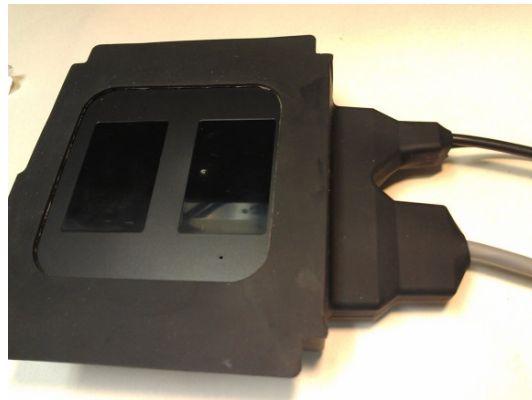
Figure 62: Terminal in Shroud
