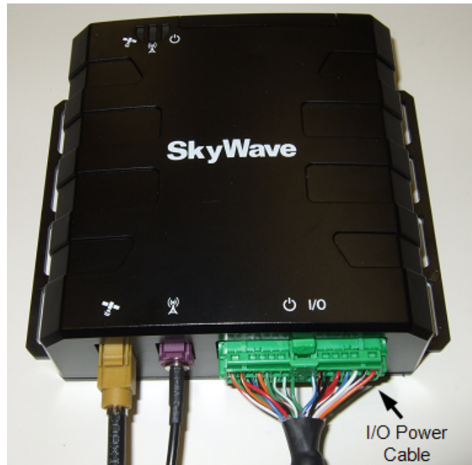
Figure 55: Connect the I/O Power Cable
