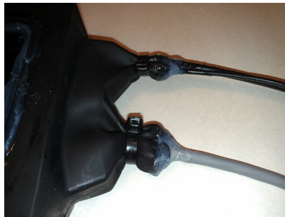
Figure 65: Cable Ties and Silicone
