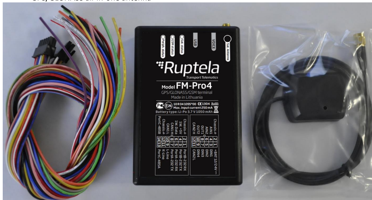
Figure 2. Box contents: FM-Pro4 device, GP/GLONASS antenna, IO cables
