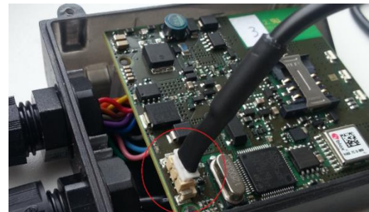
Figure 5. USB cable connection location on PCB
