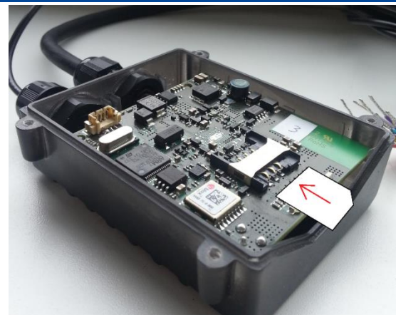
Figure 6. Insert SIM card into holder chip facing down
